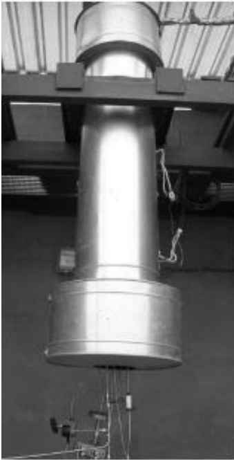
SCWO reactor and pilot demonstration plant of the High Pressure Process Group of the University of Valladolid (Spain)
