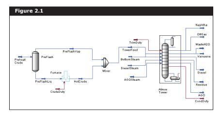
The crude column consists of a refluxed absorber with three side strippers and three cooled pump around circuits. The column sub-
